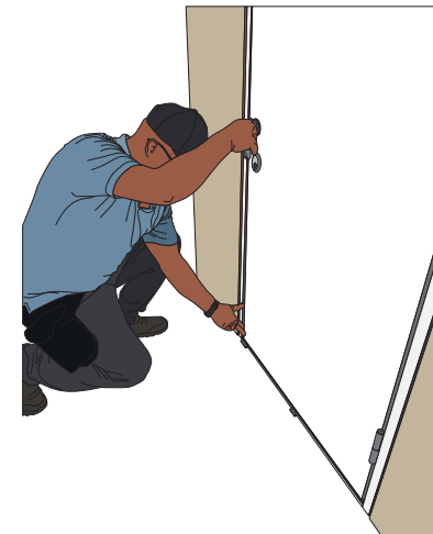
STEP 12. When both sides of the door frame are fixed in the wall opening, put the gap-appropriate pads under the middle and lock the side of the threshold.
