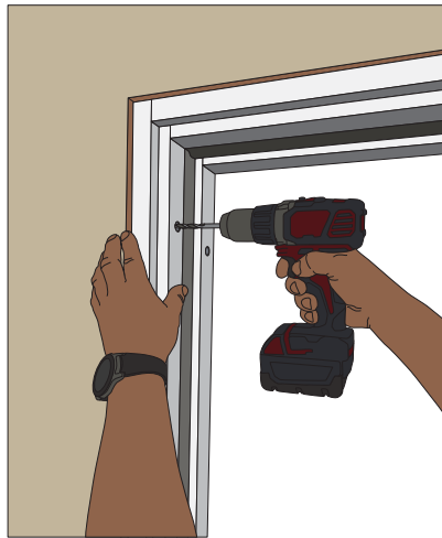
STEP 14. Fix the lock side of the door frame to the wall (drill the wall through the adjustable hole or installation bolt points in the vertical part of the door frame).
