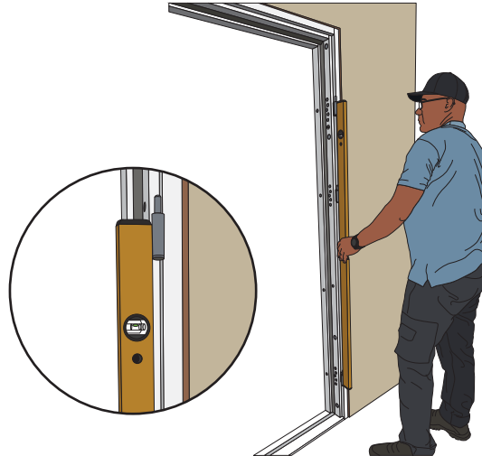
STEP 8. Double-check the fixed door frame using a level. Do the checking on the vertical hinge side inside the door frame. Make sure that all hinges are aligned on the same axis.
