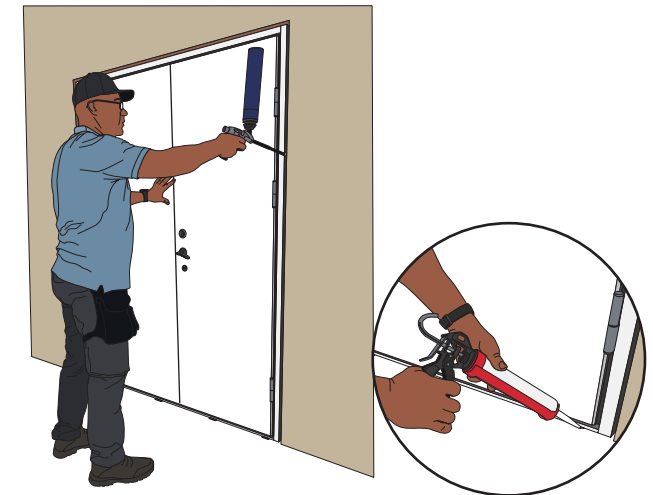
STEP 12. The gaps between the wall and the jamb are sealed with the fire resistant polyurethane foam "Penosil Premium Fire Rated B1" or with the fire resistant mineral wool class A1 or A2-s1, d0.
